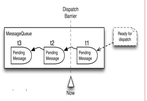
•The figure illustrates a message queue with three pending messages, sorted with timestamps where t1 < t2 < t3. Only one message has passed the dispatch barrier, i.e., the current time. Messages eligible for dispatch have a timestamp value less than the current time, i.e. "Now" in the figure.
