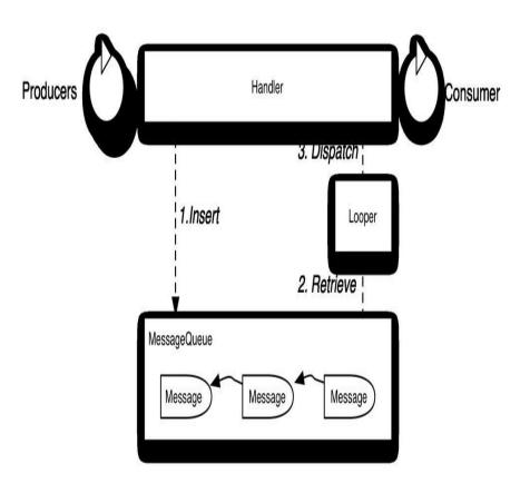
Message passing mechanism between multiple producer threads and one consumer thread. Every message refers to to the next message in the queue. Messages are inserted by producer threads and processed by the consumer thread, as illustrated in the figure.
