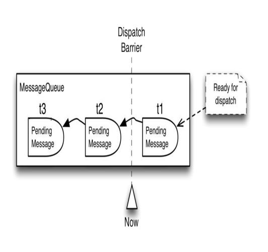
If no message has passed the dispatch barrier when the Looper is ready to retrieve the next message, the consumer thread blocks.
