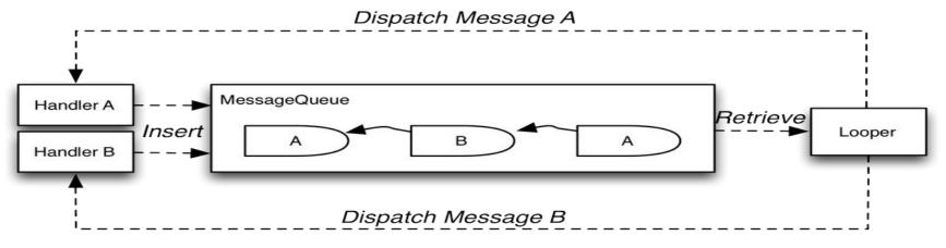
Multiple handlers using one Looper. The handler inserting a message is the same handler processing the message.
