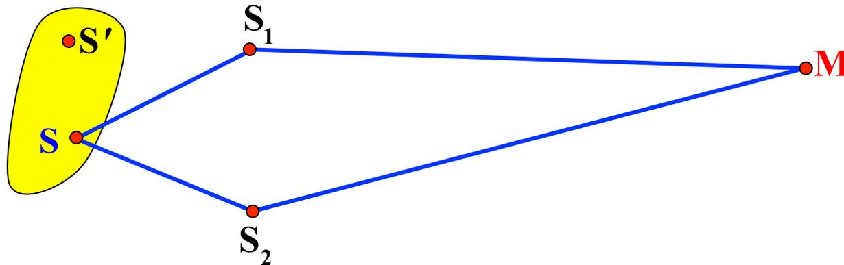
$$\begin{aligned}\Delta\delta &= \Delta[(SS_2M) - (SS_1M)] \\ &= \Delta(SS_2) - \Delta(SS_1) \\ &= (S'S_2 - S'S_1) - (SS_2 - SS_1)\end{aligned}$$
