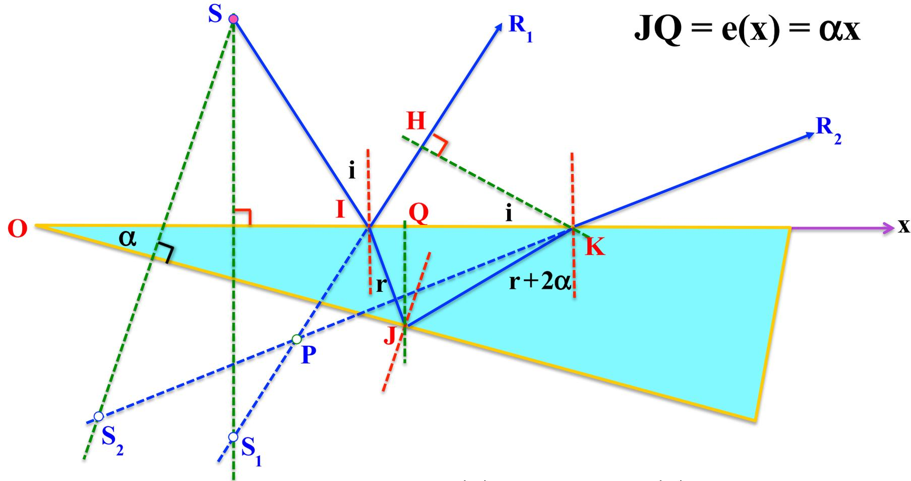
$$\delta_{\text{géo}} = L_{\text{IJK}} - L_{\text{IH}} \left\{ \begin{array}{l} L_{\text{IJK}} = n \frac{e(x)}{\cos(r)} + n \frac{e(x)}{\cos(r + 2\alpha)} \\ L_{\text{IH}} = ne(x) (\text{tg}(r) + \text{tg}(r + 2\alpha)) \sin(r) \end{array} \right.$$
