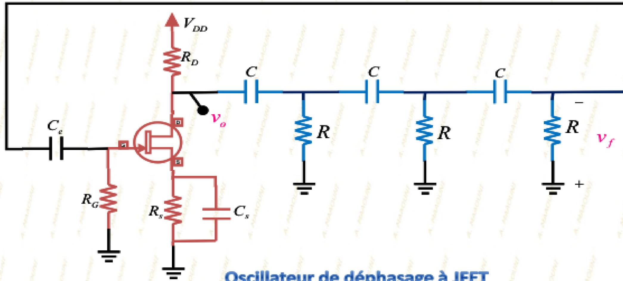
$$A = -g_m R_D \parallel r_d \cong -g_m R_D \quad (\text{si } R_D \ll r_d)$$
