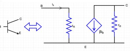
$$r_{\pi} = \frac{\beta V_T}{I_C} = 100 \frac{25mV}{1,13mA} = 2,21k\Omega.$$
